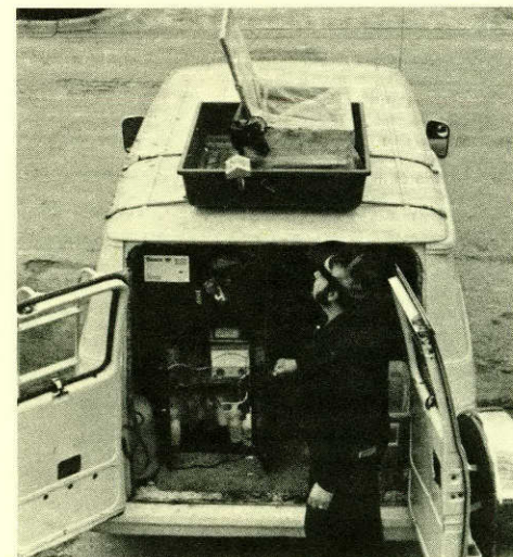
The rainfall analyzer developed by Jose Lopez-Gonzalez is housed in a van. The sampling apparatus on top automatically flips open when rain falls.
