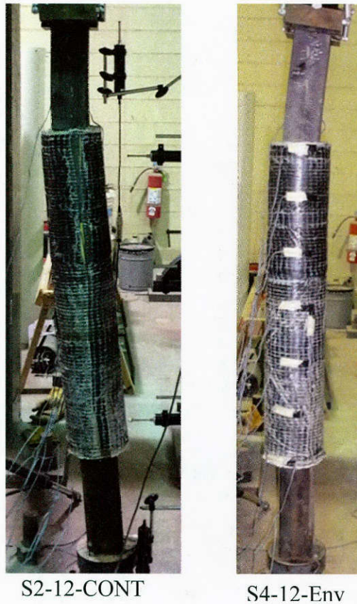
Figure 10.30: Failure of 4-in damaged piles repaired with Repair System 2 (S2-12-CONT and S2-12-Env)
