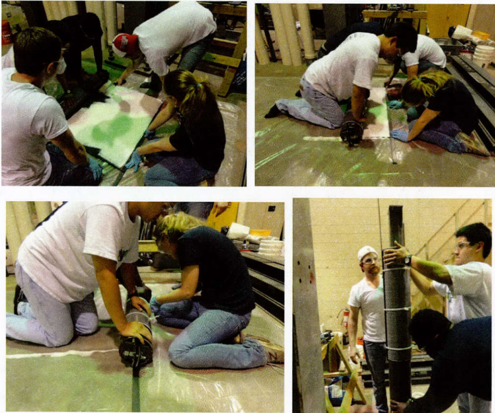
Figure 10.10: Fabrication of FRP jackets for Repair System 1
