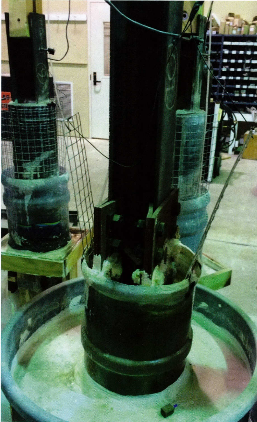
Figure 10.44: Accelerated corrosion test set-up for the piles repaired with System 3 (S3-4-Cor)
