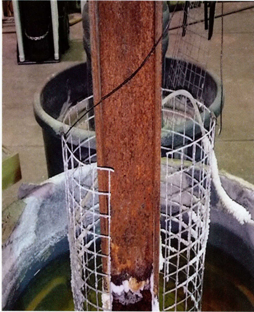
Figure 10.41: Undamaged pile (CONT-Cor) showing the rust build-up
