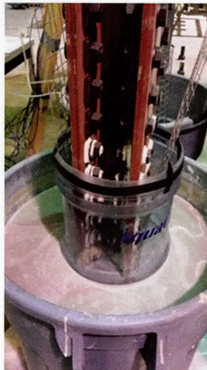
Figure 10.21: Actual set-up of accelerated corrosion process
