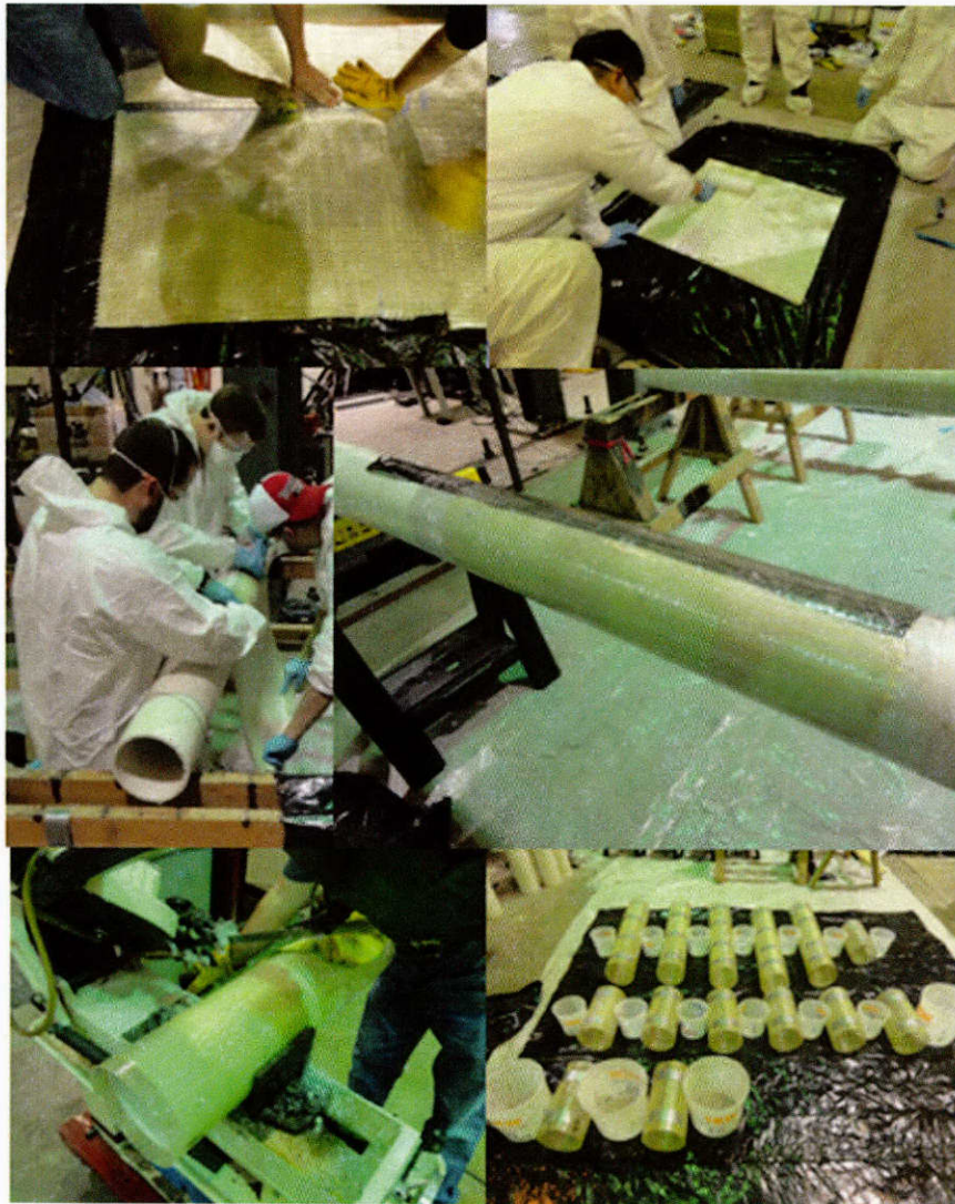
Figure 10.13: Fabrication of cylindrical GFRP shells
