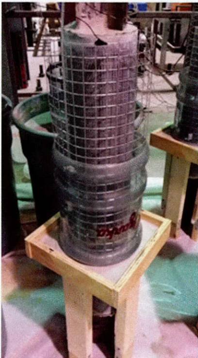
Figure 10.21: Actual set-up of accelerated corrosion process
