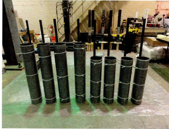
Figure 10.11: Fabricated FRP jackets for Repair System 1
