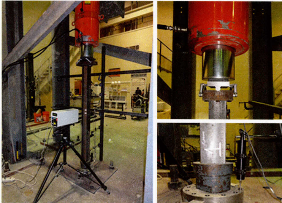
Figure 10.24: Actual test set-up for failure testing
