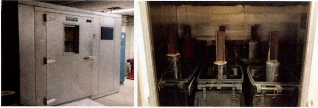
Figure 10.18: Environmental chamber and the small-scale test piles placed inside
