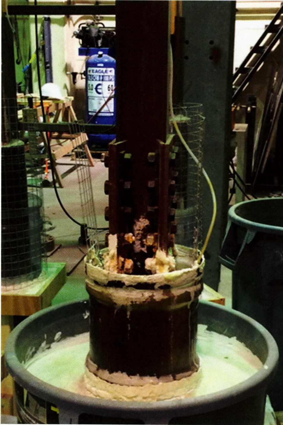
Figure 10.47: Accelerated corrosion test set up for Repair System 3 (S3-12-Cor)
