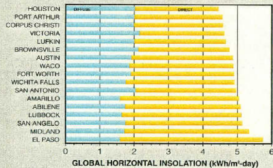
FIGURE 3. Global Horizontal Insolation for Texas Cities. Throughout Texas, sunshine is adequate to power rooftop systems such as photovoltaic or water heating systems.
