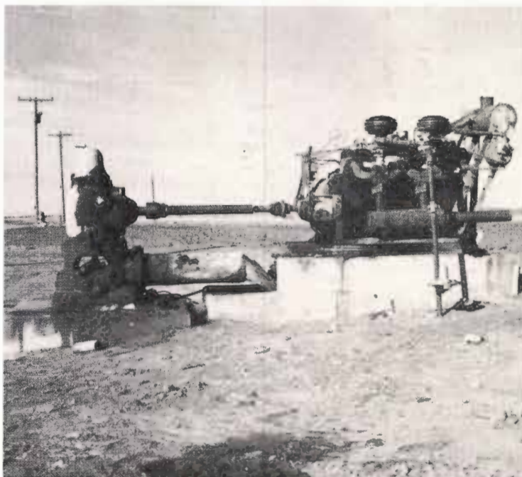
At left, above, is pictured a typical irrigation well operating in the southern High Plains of Texas without a guard covering the high speed drive shaft between the engine and
