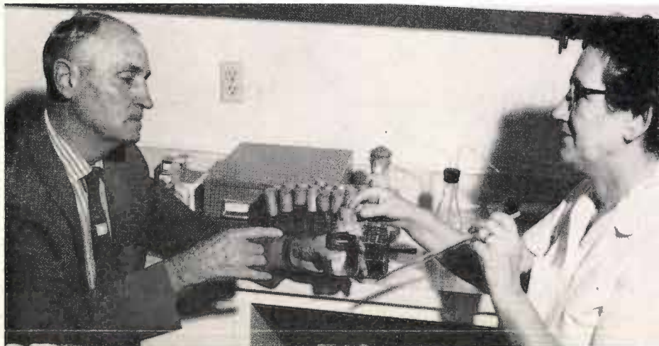
Mrs. Ray Chaney, Lubbock Health Unit Laboratory Assistant, prepares to analyze a sample of water taken from a domestic well by W. R. Bradford. She will check the water for coliform organisms which, if present, will indicate contamination.
