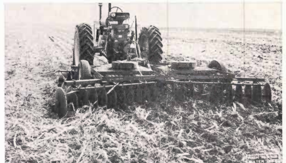
Grain sorghum stubble is another readily available source of humus. The disc plow is shown above as it mulches the stubble into the soil.
