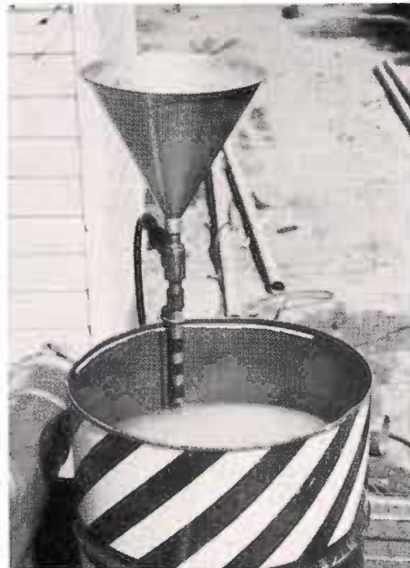
Separan AP-30, a powdered flocculating chemical is mixed with water at a ratio of 2 pounds to 55 gallons.
