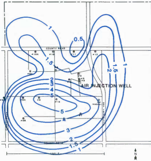
CHANGES IN WATER LEVELS - IDALOU TEST SITE JUNE 26, 1982 TO SEPTEMBER 30, 1982 (CONTOURED IN FEET) INCREASED VOLUME OF WATER IN STORAGE = 371.33 ACRE/FEET
