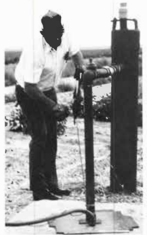
STEEL TAPE IN HAND , Obbie Goolsby, Water District Engineer Technician, measured the depth-to-water in this well. Only a small hole is needed to feed the steel tape marked with carpenter's chalk through the pump base until it reaches the static water level in the well. These measurements help the Water District staff keep a close eye on the effects of yearly pumpage of water from the underlying formation.
