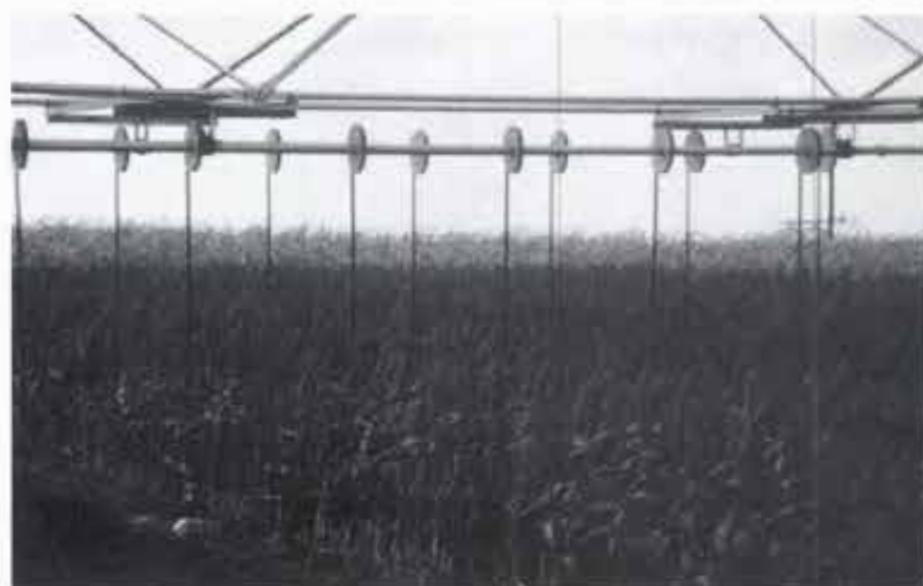
CHEMIGATION is accomplished through the new MFIS sprinkler system designed for simultaneous irrigation and chemical application.
