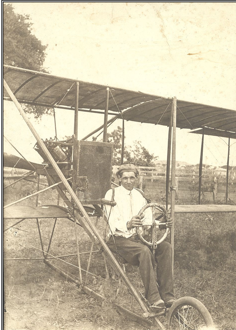
The first airplane at Kerrville, Texas, during the Kerr County Fair on the old Fairground in Westland, date 1913, airplane Curtis Pusher. The pilot, name unknown, was a Frenchman. The plane was shipped in on a railroad car and assembled at the Fairground. Picture was taken by E. T. Butt of Kerrville, now with Post Office here.
