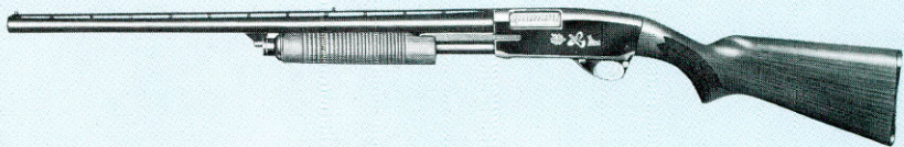
Savage m/30-L shotgun with left ejection port.
