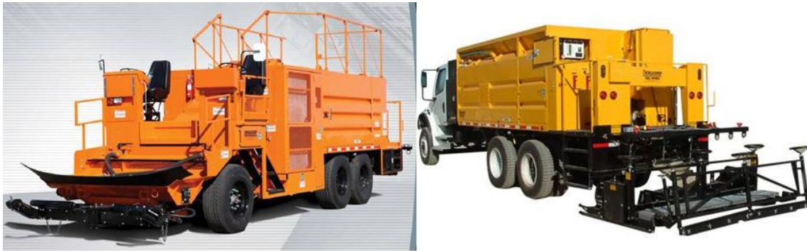
Figure 4-1. Self-Propelled Unit (Left) vs. Truck-Mounted Unit (Right).
