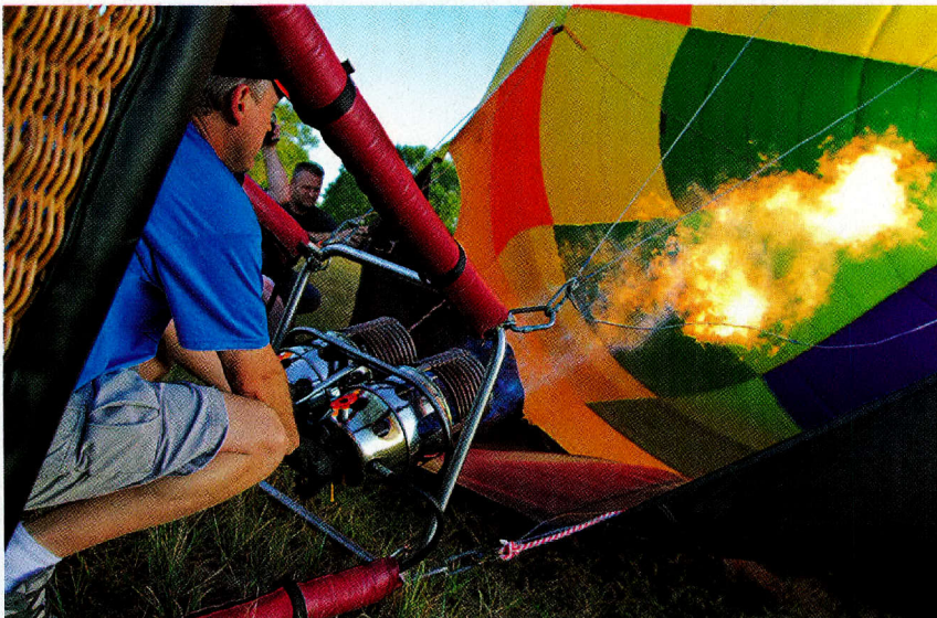
ABOVE: With his hot air balloon, Sundance , already about two-thirds full, balloonist Rick James of Judson blasts the propane burners to fully inflate the envelope. RIGHT: Sundance flies overhead during the Great Texas Balloon Race.
