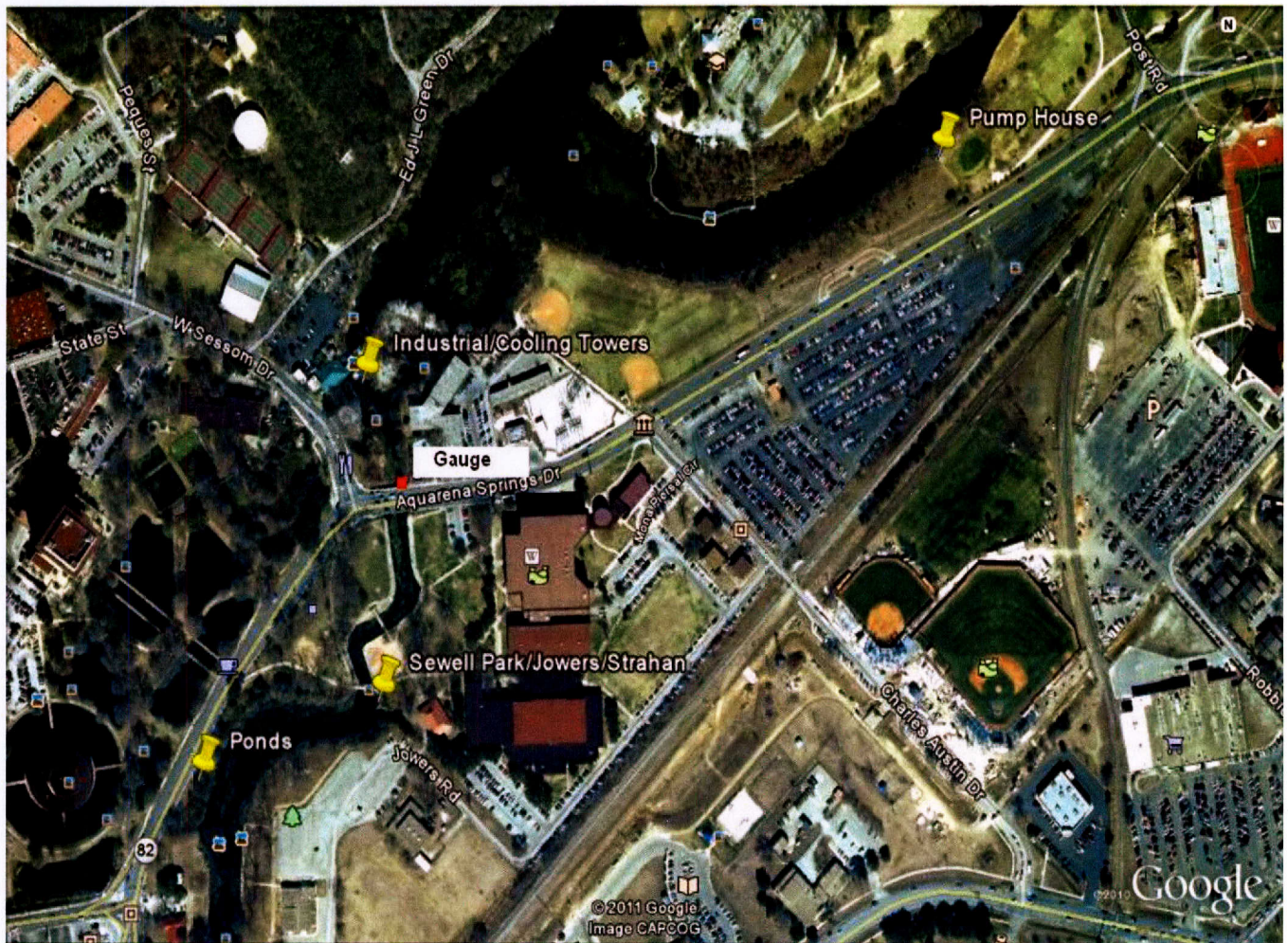
Figure 5-3. Texas State University Surface Water Diversions. The diversions are identified with stick pins. The diversions at the pump house (slough arm of Spring Lake) and industrial cooling towers are permitted under TCEQ Certificate 18-3865. The 513 ac-ft/yr municipal water right has not been exercised, and no diversion for this right currently exists. The diversions at Sewell Park and the “ponds” are permitted under TCEQ Certificate 18-3866. (See Sections 2.5.5.1 and 2.5.5.2 respectively).
